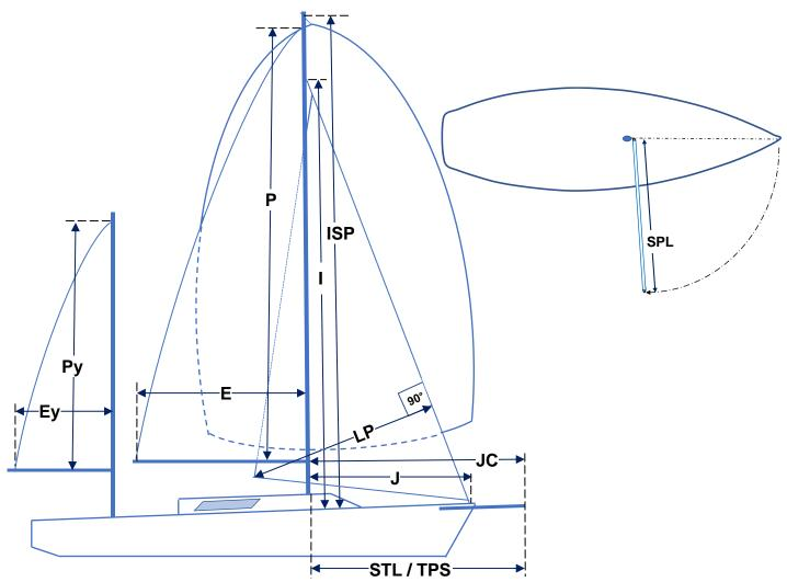
I Dimension measured from the sheer line at the mast to the maximum hoist
